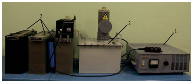
Fig. 1. An electric pulse plant. 1 – a control panel, 2 – a generator with a discharger, 3 – a protection unit with a capacitor
