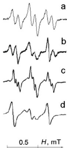
Fig. 3. EPR spectra of a mixture of I and anabasine in toluene solution at 310 (a), 255 (b), 238 (c), and 183 K (d). [Y] = 0.04 mol/L.
