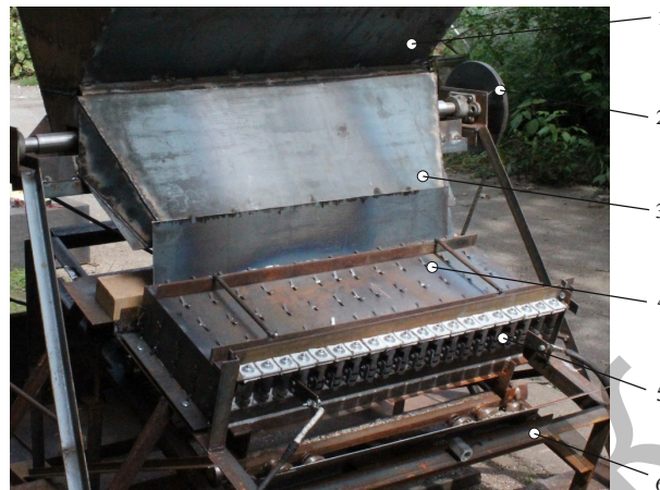
Figure 1. Furnace prototype with a vibrating base plate: 1 is the drum doser; 2 is the doser drive; 3 is the trigger tray; 4 is the thermal lid; 5 is the heating system; 6 is the frame
